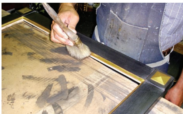
A finisher applying a stippled patina on the gold front cove.
